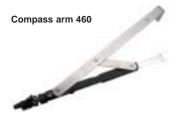
USE For tilt-and-turn windows. Compass arm 300 on frames of width 375÷554 mm, and height 530÷2400 mm. Compass arm 460 on frames of width 555÷1700 mm, and height 530÷2400 mm. For width of 1200÷1700, the additional compass arm item T1107 or T1407 is to be STANDARD EQUIPMENT
